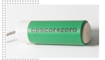
The zinc metallic element is in contact with a solid electrolyte, whose special composition ensures permanent active conditions of the zinc, preventing the formation of passive layer (Patent Application N. 102015000021001).
