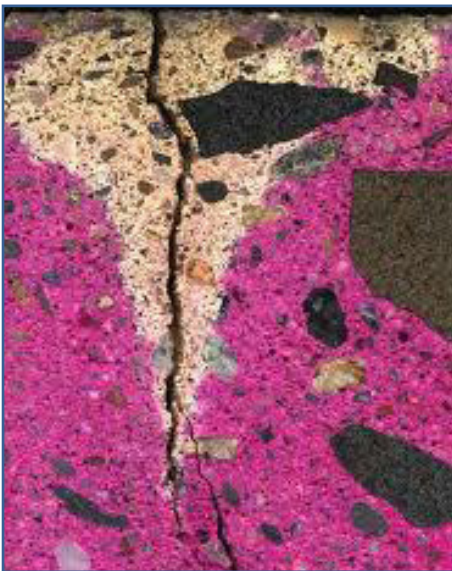
Fig. 3 - Carbonation test of concrete with phenolphthalein
