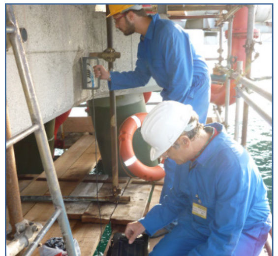
Fig. 6 - Concrete resistivity measurements
