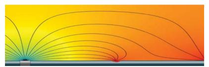
Finite Element Methods (FEM) are used to model the electrical field around the pipeline and close to coating defects. Modelling allows to correctly interpret the inspection results. In case of buried pipelines, the electrical field is modelled considering the burial depth and the sea mud resistivity.
